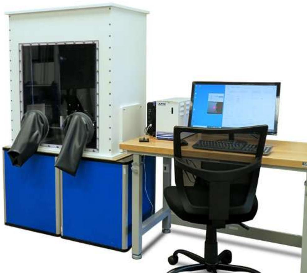
For customers who need to scan samples in an oxygen-free environment, the HR-2D AFM in a glove box is the ideal product.
