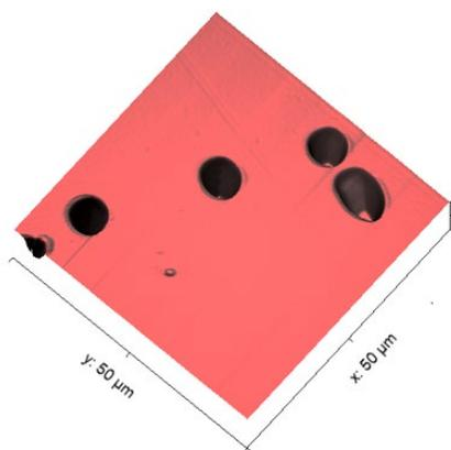
Kimberly's three dimensional image of the pores in a plastic filter.
