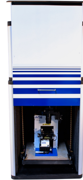
TT-2 AFM supported on a platform that is suspended by bungee cords.
