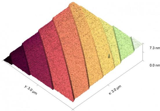
*Figure 1a: Three dimensional color scaled image of SiC. The steps on this sample are 750 pico-meters*
