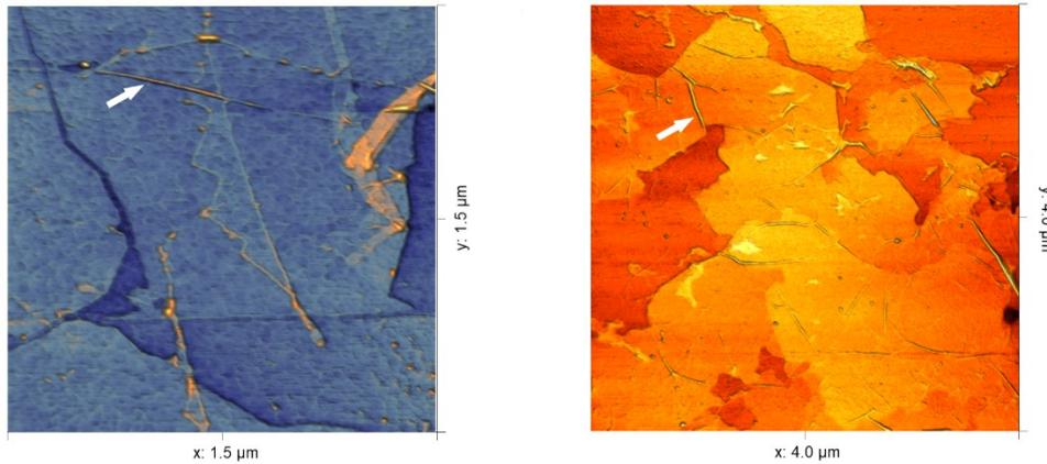
*Figure 2. Examples of AFM images of CVD graphene deposited on Si/SiO<sub>2</sub> wafers. Left: Single-layer graphene on a silicon wafer. In this example, the effect of the underlying texture on the graphene sheet is clearly seen. Right: Multilayer graphene of a silicon wafer. Arrows highlight some defects, typical of CVD graphene.*
