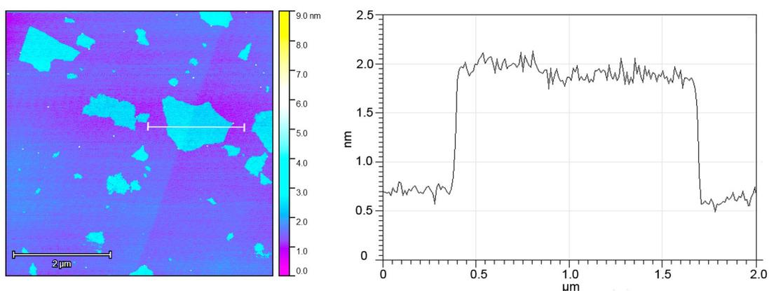
*Figure 4. Height image of single graphene flakes on a well-polished silicon wafer sample, and height profile across the indicated flake.*
