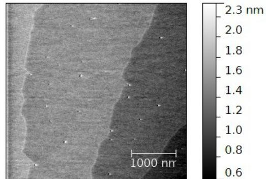
*Figure 1b: Gray scale image of Si(111) atomic steps. The steps on this sample are 300 pico-meters in height.*
