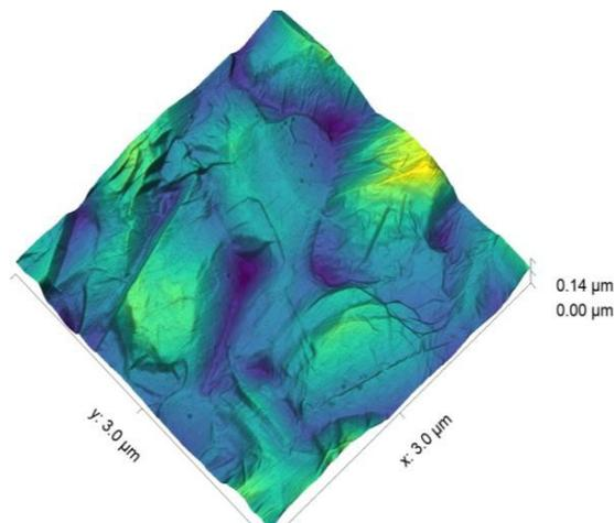
*Figure 3. Image of multi-crystalline nickel film with graphene deposited on top: This image shows the surface had almost 100% coverage; However after transfer to another substrate much lower coverage was found.*
